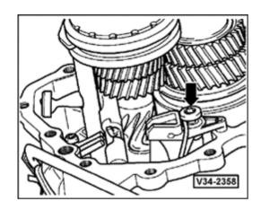
Then unbolt the detent segment (arrow) and swing it out.
