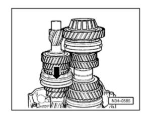
Turn transmission housing and engage 3rd gear (direction of arrow).
