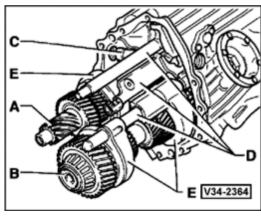
The input shaft -A-, the pinion shaft -B-, the relay shaft -C-, the selector rods -D-with selector shaft and the selector forks -E- must be carefully pulled out together.
